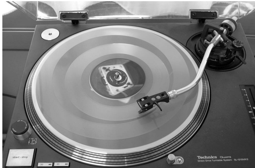
Fig. 2: Janek Schaefer, On/Off LP (2001). Single-sided LP record with two grooves: one centric, one eccentric. Originally intended to be played on a turntable with two pickup systems.
